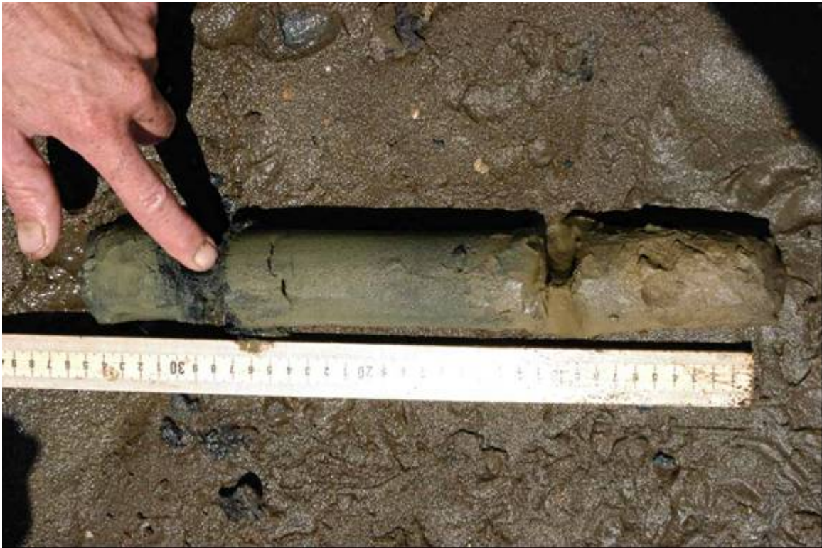
Figure20. Sediment core at South R. Farm Park, June 2004 showing 5-6 cm over the old black organic marsh layer.
