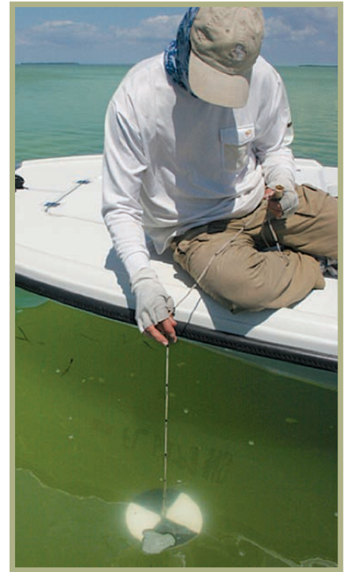
Figure 36. Using a secchi disk to measure water clarity.
